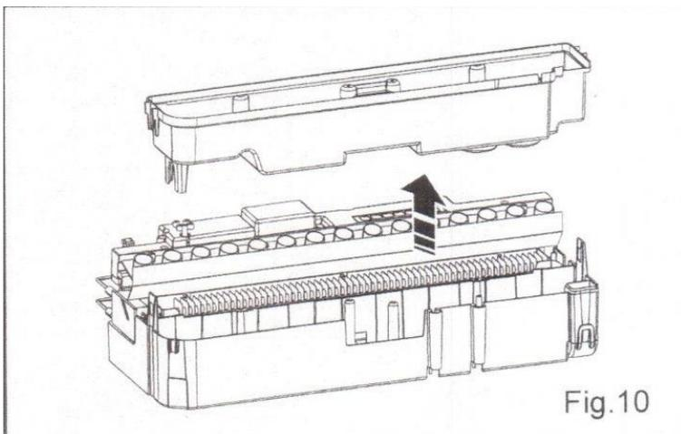
7. Carefully empty the sump into the sink taking note that the transducer is held in place by a retaining clip.
